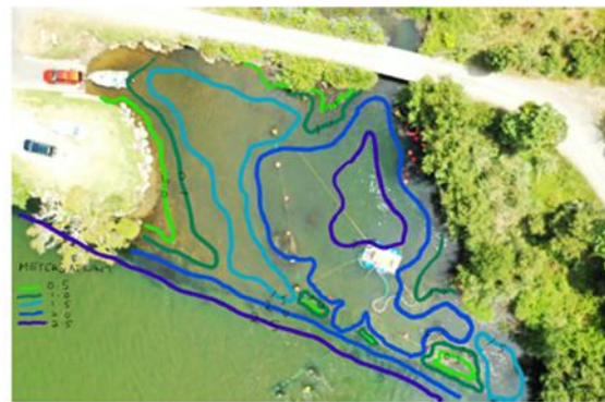
Fig 5: Depth contours (approx.) of Bell Road site after dredging works
