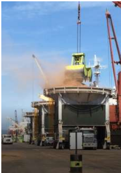
Video 1 Dust generated from overfilled hopper, overfilled trucks and excessive wind during palm kernel unloading [Mount Maunganui Wharves 12:31 PM 17 Oct 2016. If reading electronically use control click to view, alternatively go to: https://drive.google.com/open?id=0ByQyNZDMNCDA3NiVjRETWk1NGs ]
