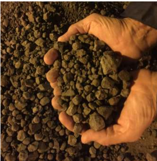
Photo 3 Clinker collected from wharf during unloading [Mount Maunganui Wharves 5:29 AM 21 Oct 2016]
