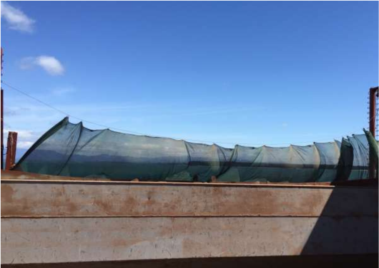
Photo 20 Wind break (nets) on windward side of boat during unloading of palm kernel. [Sen Treasure, Mt Maunganui Wharves, 11:48 AM 18 Oct 2016]
