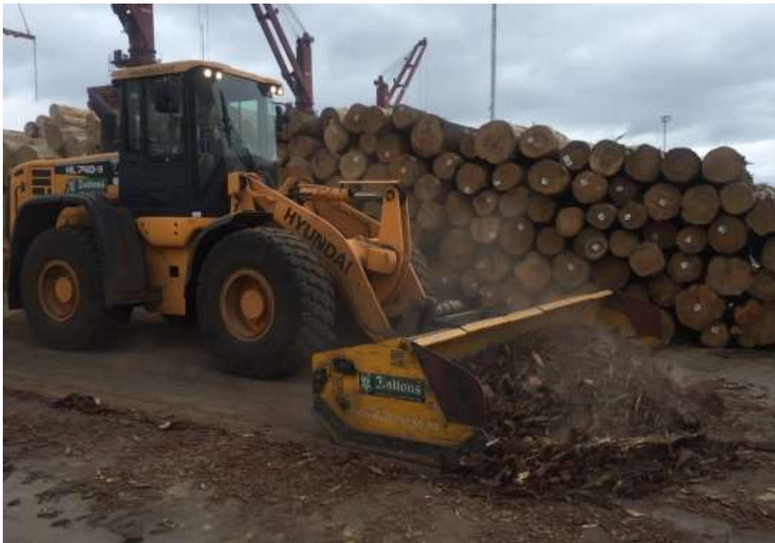
Photo 9 Daltons scraping bark debris (under contract to Port of Tauranga) [Mt Maunganui Wharves 12:06 AM 20 Oct 2016]
