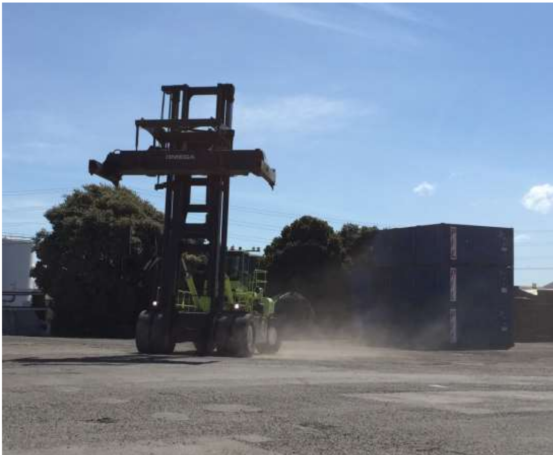
Photo 7 Dust arising from vehicle movements over sealed surface [Container storage area on Waimarie Street, Mount Maunganui Wharves, 2:48 PM 17 Oct 2016 ]
