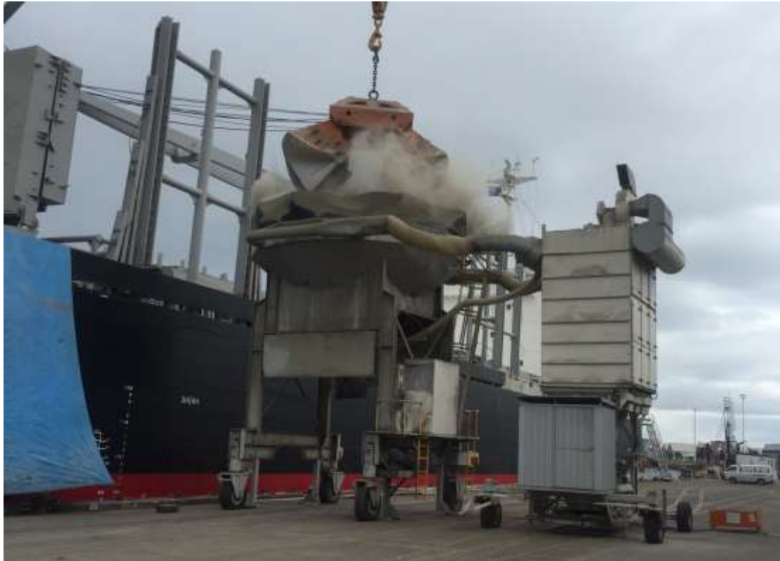
Photo 4 Clinker unloading using dedicated hopper and bag filter [Mount Maunganui Wharves 11:49 AM 20 Oct 2016]
