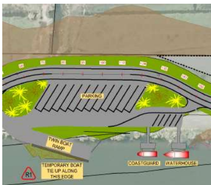
Figure 7 New boat ramp, moorings, carpark and realigned Ford Rd
