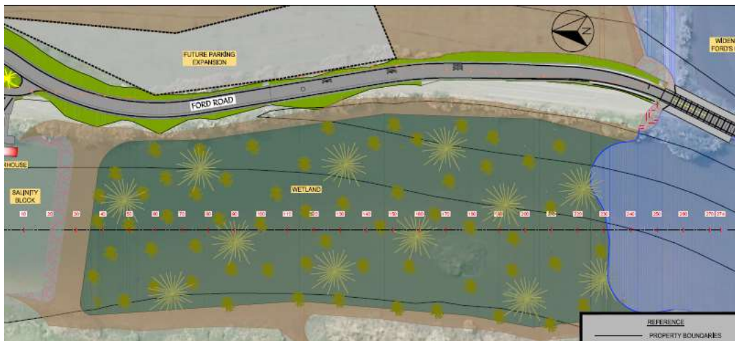
Figure 8 Closure of Ford Loop Channel showing salinity block and wetland
