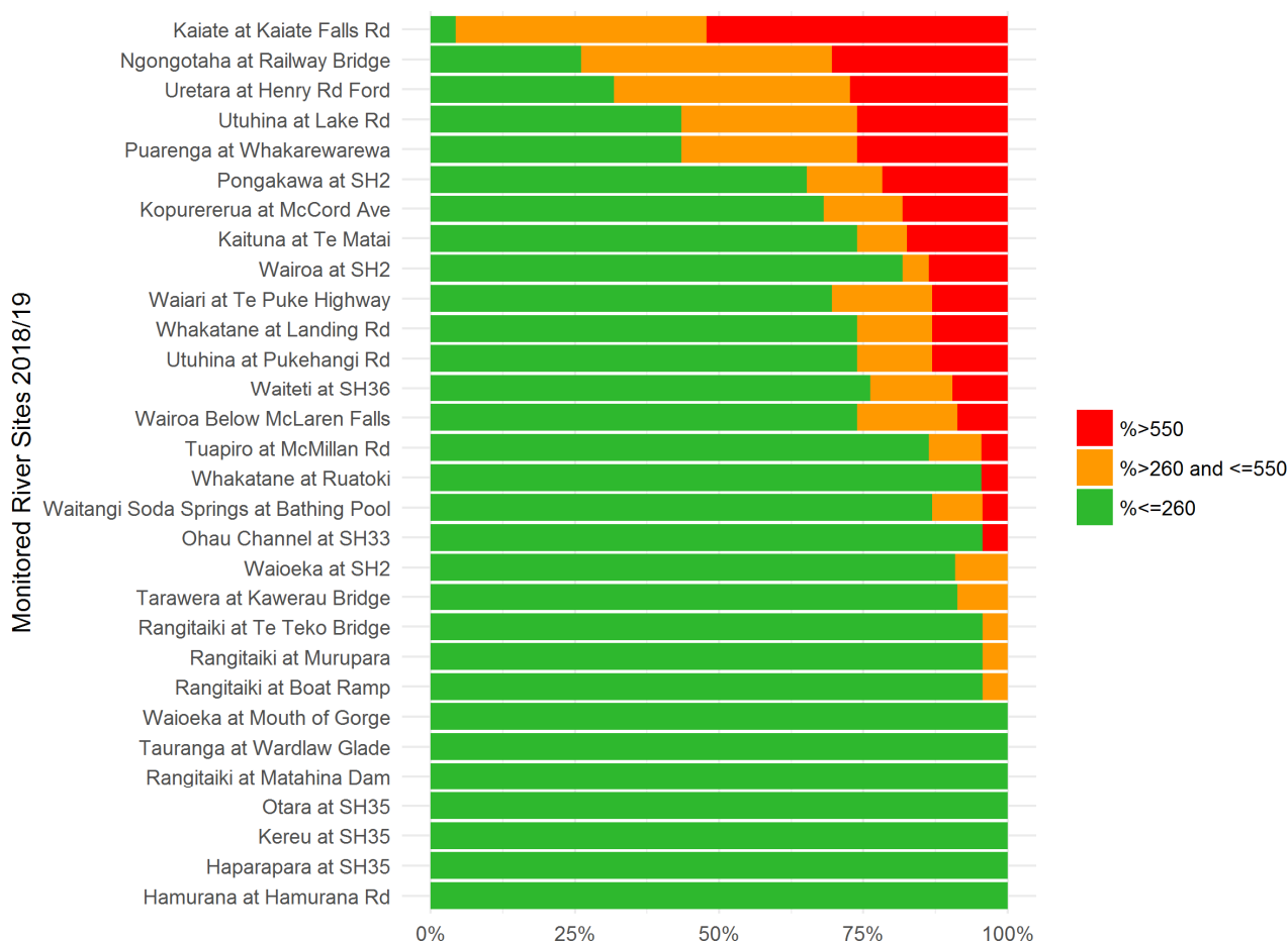
Figure 3.3 Percentage of samples from river and stream sites with E. coli concentrations (cfu/100ml) in each of the modes in the Microbial Water Quality Guidelines (MfE, 2003), 2018/19 bathing season.
