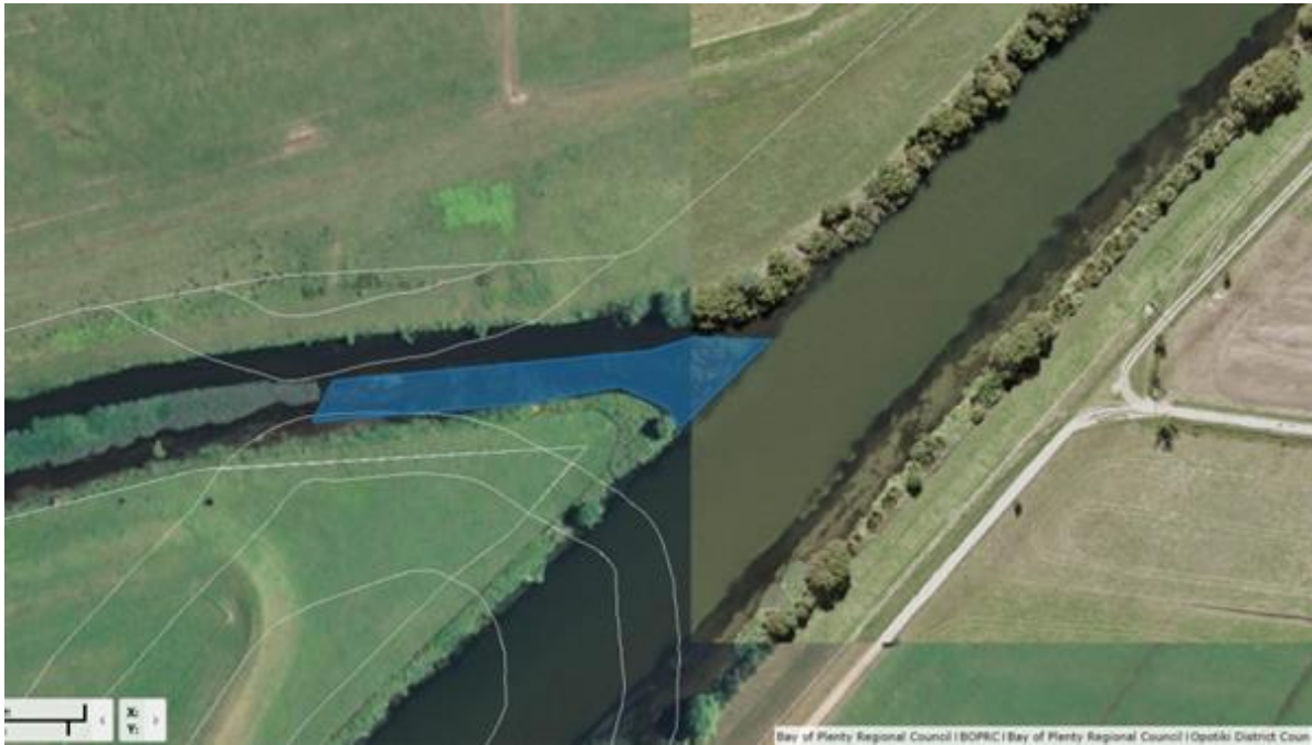
Figure 2: Kopuaroa Canal Dredging Extent
