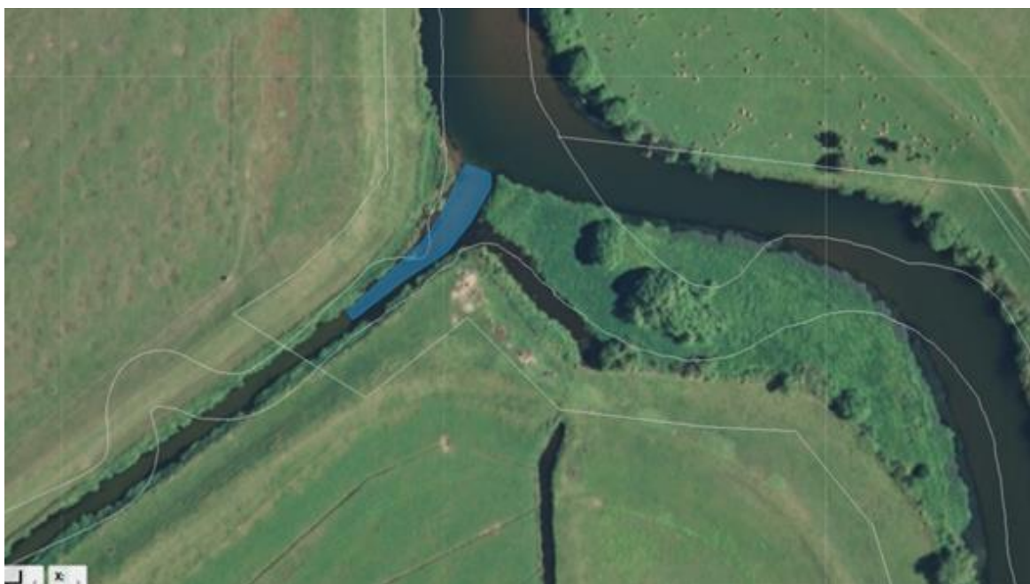
Figure 4: Waiari Canal Dredging Extent
