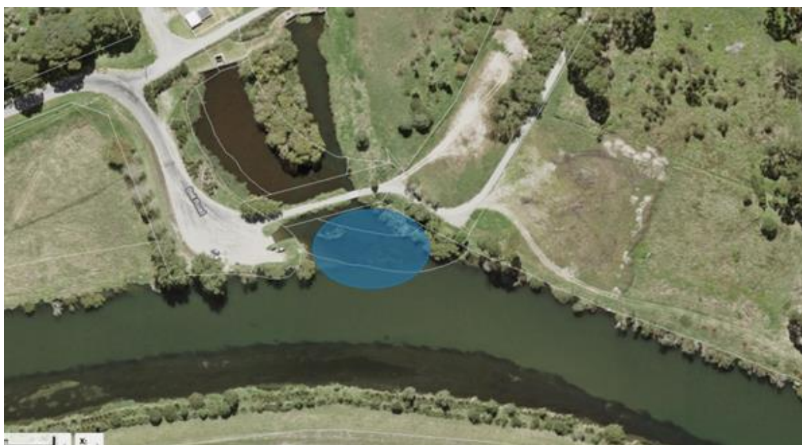
Figure 1: Bell Road Drain Outlet Dredging Extent
