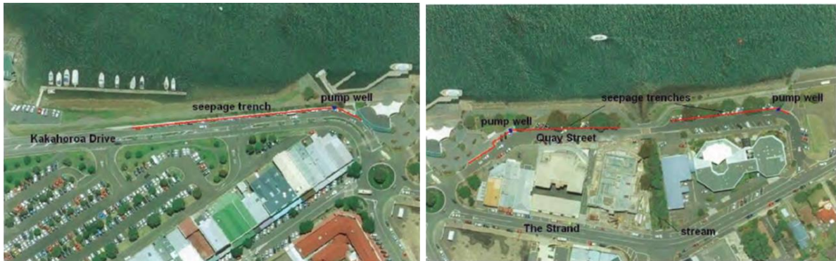
Figure 2: Proposed locations of seepage trenches
