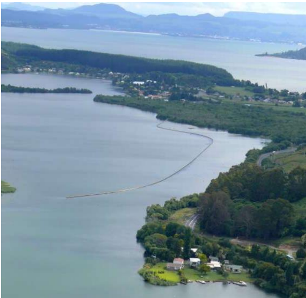
Figure 3. Photo of Lake Rotoiti (foreground) and Lake Rotorua showing the Ohau Channel diversion wall which directs water toward the Kaituna River outflow of Lake Rotoiti (foreground) and away from the main basin of the lake (left-hand side). Photo: Andy Bruere.
