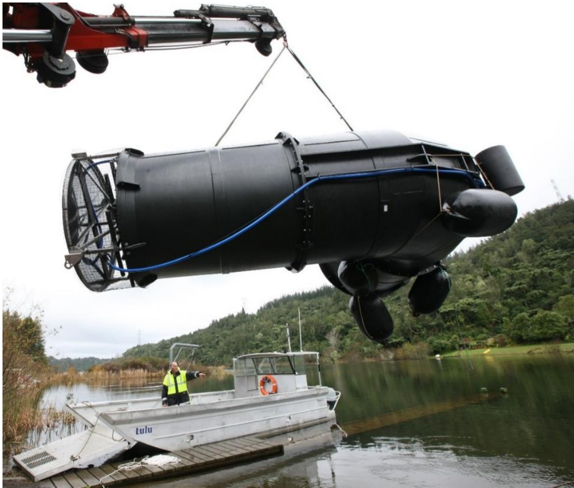
Figure 6. Commissioning of a destratification device designed to fully mix the water column using air-lift of bottom waters. Photo: D. Hamilton.
