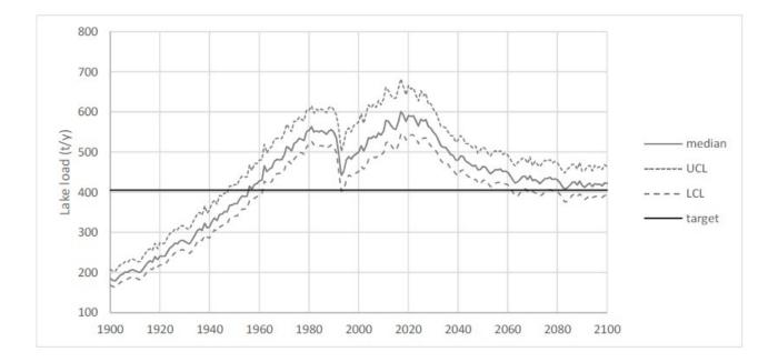
Figure 16 Predicted lake loads 1900-2100. From 2010 staged reductions in nitrogen loss are modelled. Results show the 'most likely' (median) loads together with approximate upper (UCL) and lower (LCL) bounds. The 'target' of 405 t y-1 excludes rain falling directly on the lake (Figure 3-11 reproduced from Rutherford and MacCormick 2016).
