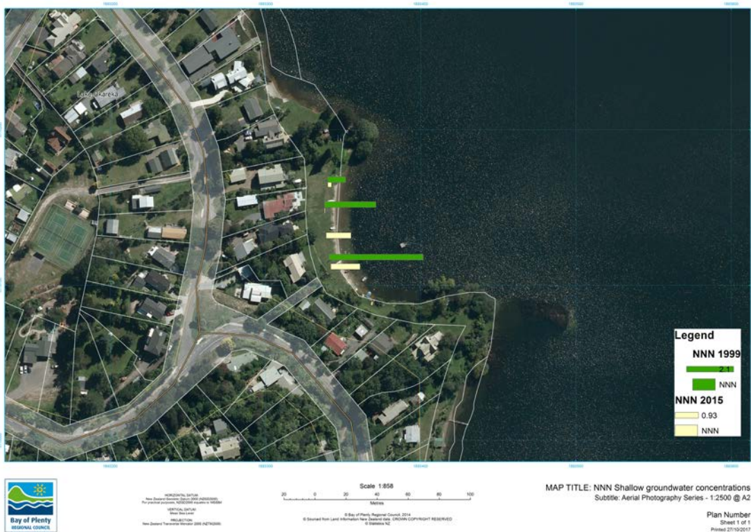
Figure 4.1.2 Shallow groundwater nitrate-nitrogen concentrations, Steep Street beach. Green bars are from NIWA study 1999, yellow bars are from 2015.
