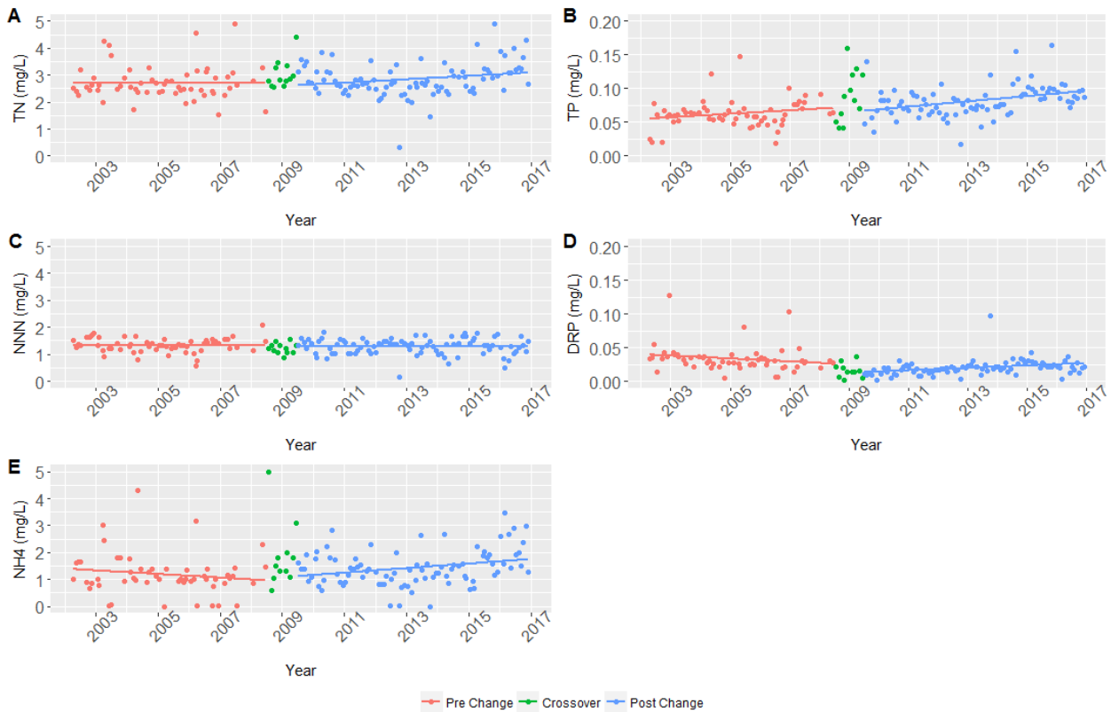
Figure 45 Trend plots for TN, TP, NNN, DRP, and NH4-N (A-E) at the Waiohewa at Rangiteaorere Road water quality site, for the period of 1 January 2002 to 31 December 2016. Plots are based on unadjusted data, split into pre (red) and post (blue) lab method change groups, with a one year crossover period (green). Pre and post lab method groups include a fitted linear regression model.
