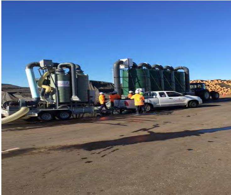
Image 1: Genera workers apply recapture technology to log stacks
