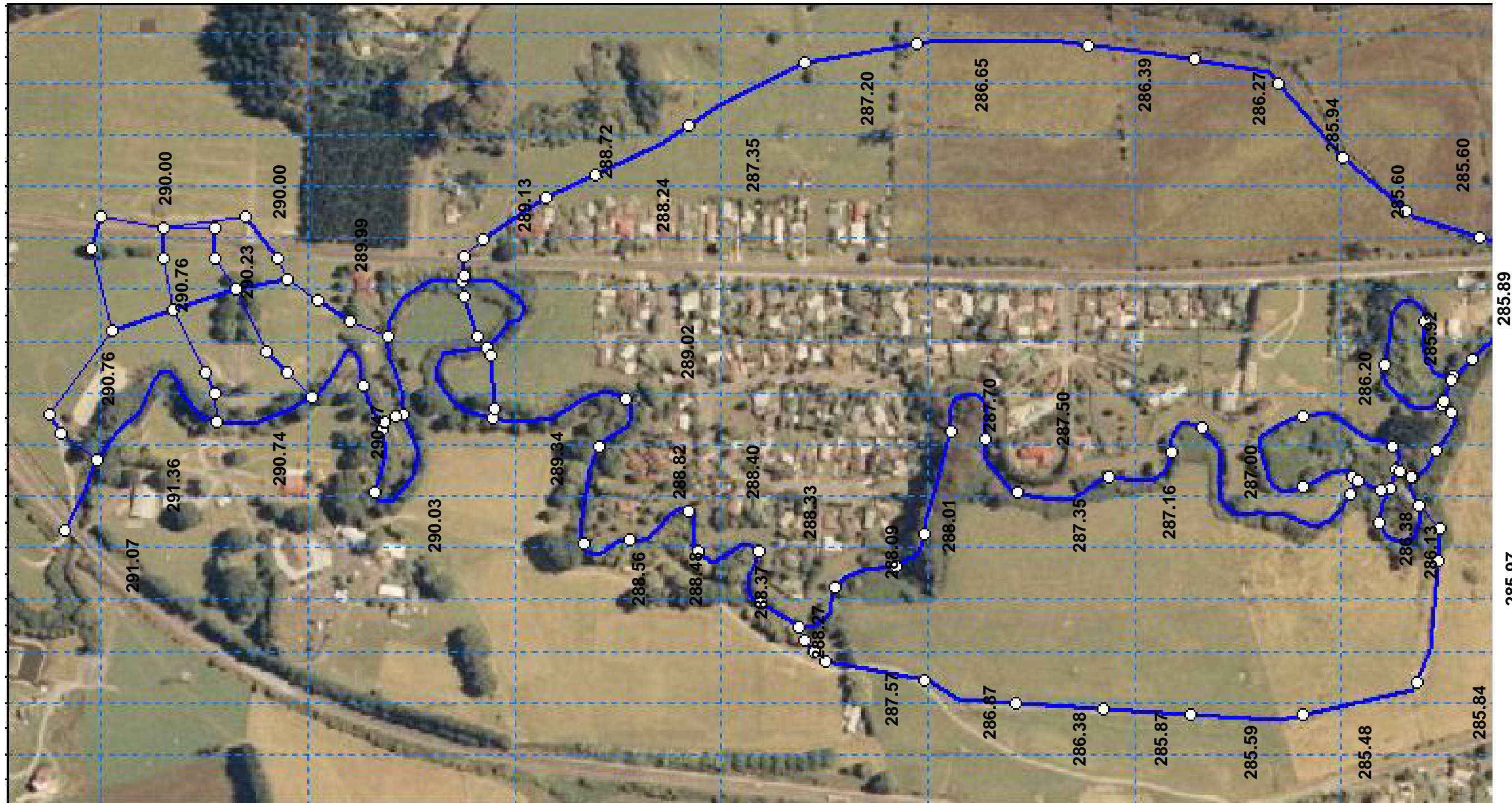
Figure 9 1% Annual Exceedence Probability Flood Levels for Ngongotaha Stream and Floodplains Inclusive of Freeboard – Upstream Area
