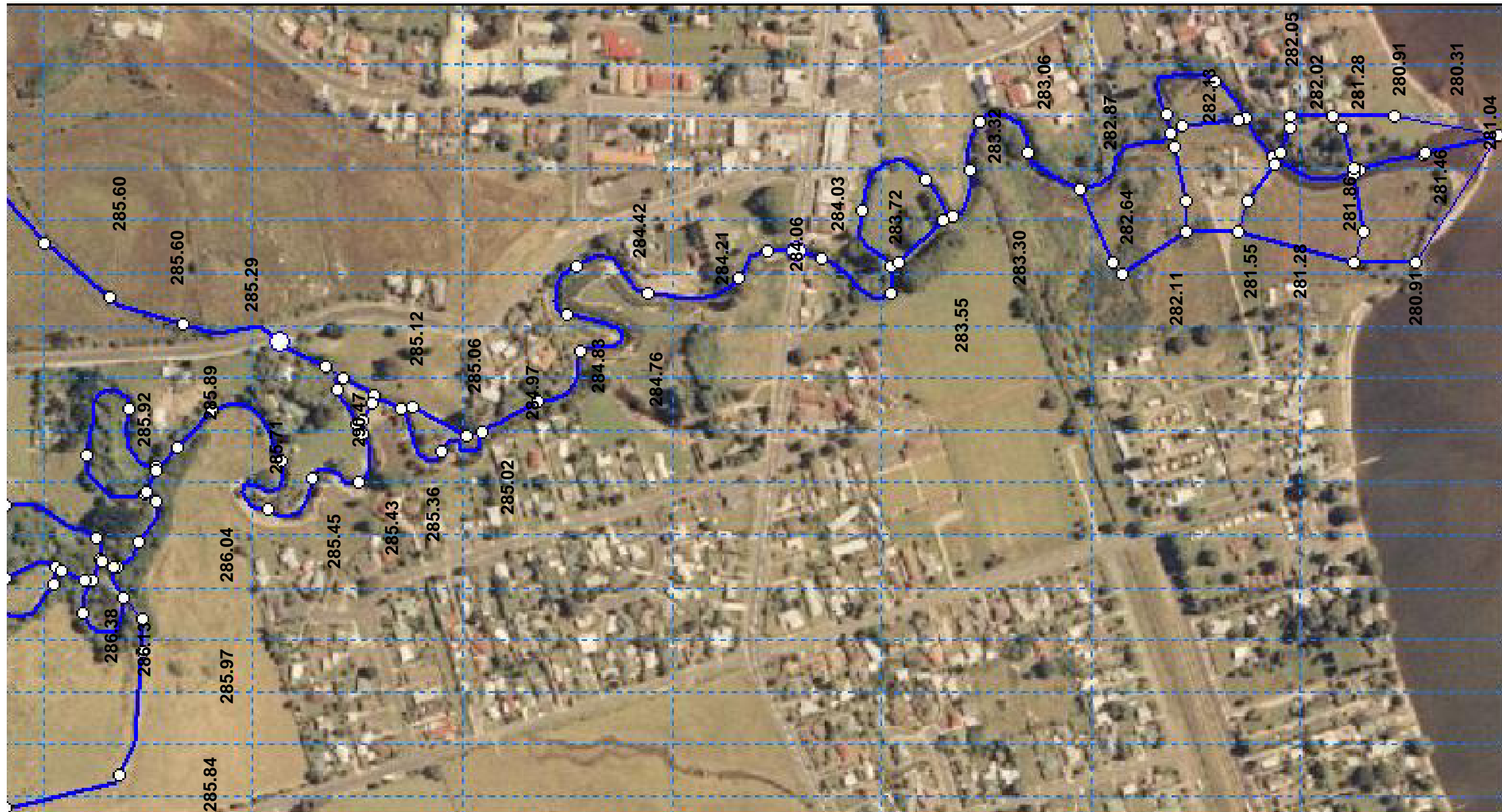
Figure 10 1% Annual Exceedence Probability Flood Levels for Ngongotaha Stream and Floodplains Inclusive of Freeboard – Downstream Area
