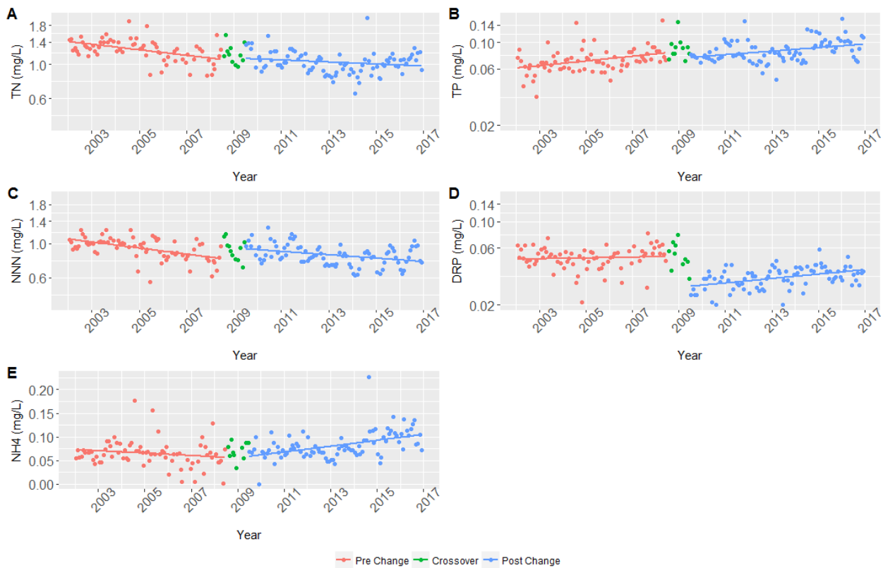
Figure 27 Trend plots for TN, TP, NNN, DRP, and NH4-N (A-E) at the Puarenga at FRI water quality site, for the period of 1 January 2002 to 31 December 2016. Plots are based on unadjusted data, split into pre (red) and post (blue) lab method change groups, with a one year crossover period (green). Pre and post lab method groups include a fitted linear regression model. TN, NNN, TP, and DRP are plotted on log transformed axes.
