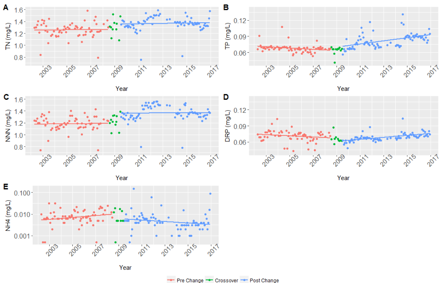
Figure 13 Trend plots for TN, TP, NNN, DRP, and NH 4 -N (A-E) at the Awahou at SH 36 water quality site, for the period of 1 January 2002 to 31 December 2016. Plots are based on unadjusted data, split into pre (red) and post (blue) lab method change groups, with a one year crossover period (green). Pre and post lab method groups include a fitted linear regression model. NH 4 -N is plotted on a log transformed axis.
