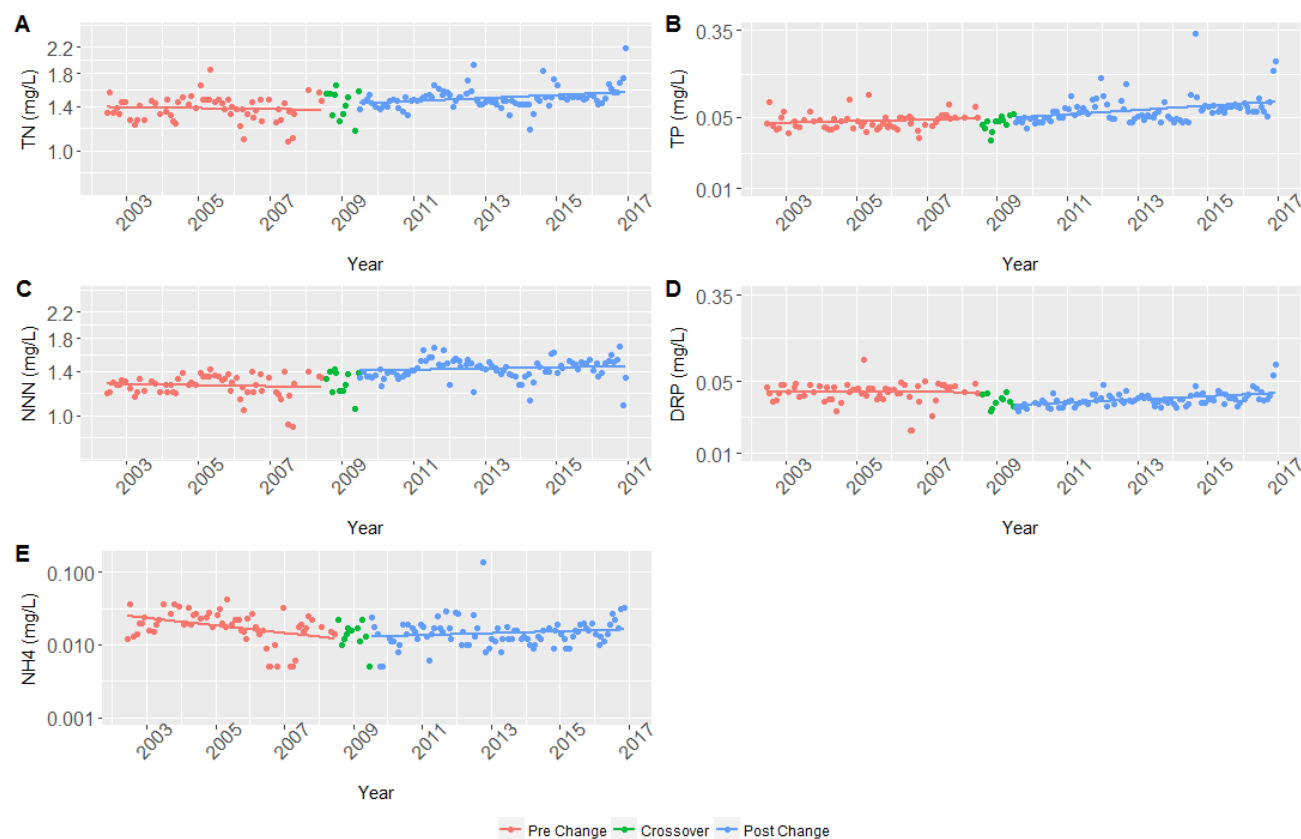
Figure 53 Trend plots for TN, TP, NNN, DRP, and NH4-N (A-E) at the Waitetī at SH 36 water quality site, for the period of 1 January 2002 to 31 December 2016. Plots are based on unadjusted data, split into pre (red) and post (blue) lab method change groups, with a one year crossover period (green). Pre and post lab method groups include a fitted linear regression model. TN, NNN, NH4-N, TP, and DRP are plotted on log transformed axes.
