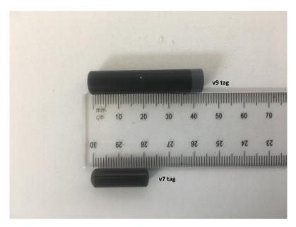
Range testing of the tags is underway. This will tell us how spread the receivers should/can be around the lake. Shortly, a small tag retention trial will begin to ensure catfish do not reject the tags. This is an important step before we begin the field trial as catfish are notorious at rejecting tags.
