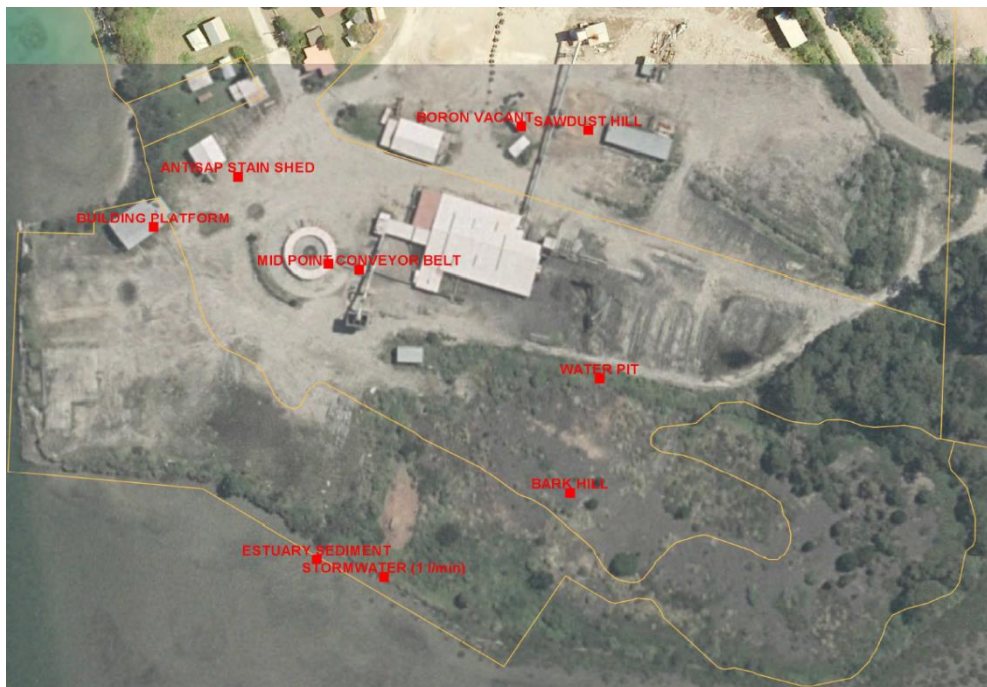
Figure 2: Soil, stormwater and sediment sampling locations associated with the 2011 BoPRC site investigation.
