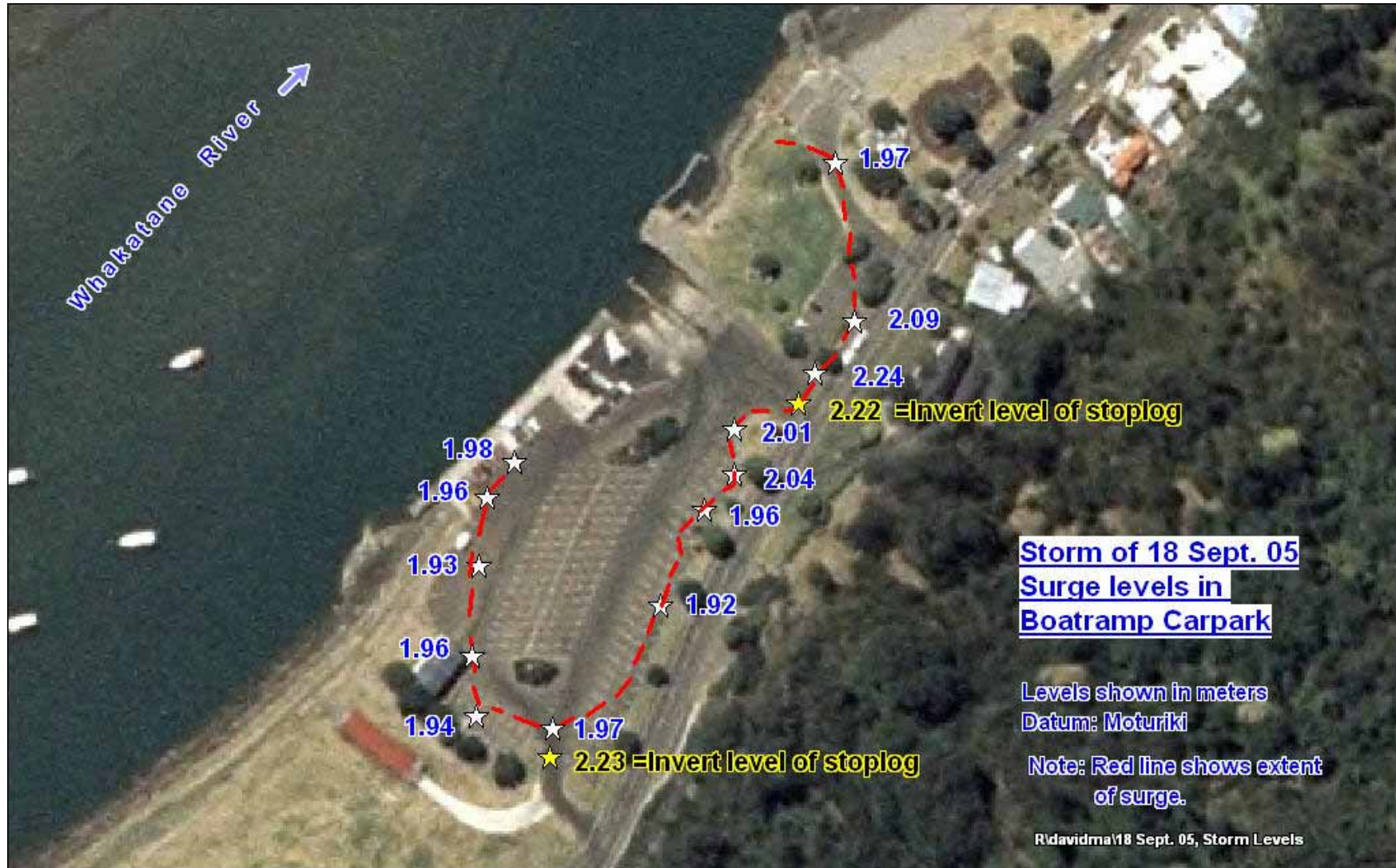
Figure 2 Debris levels reached in the Whakatane River Boat Ramp car park.
