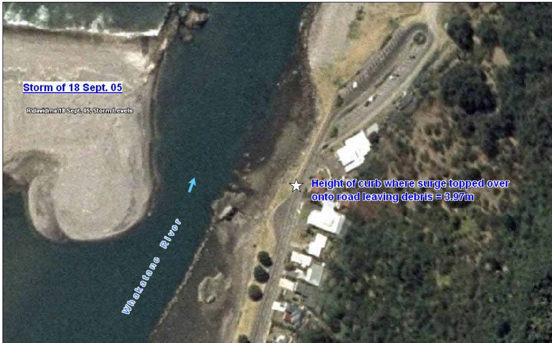
Figure 3 Debris levels reached in the Whakatane River entrance.
