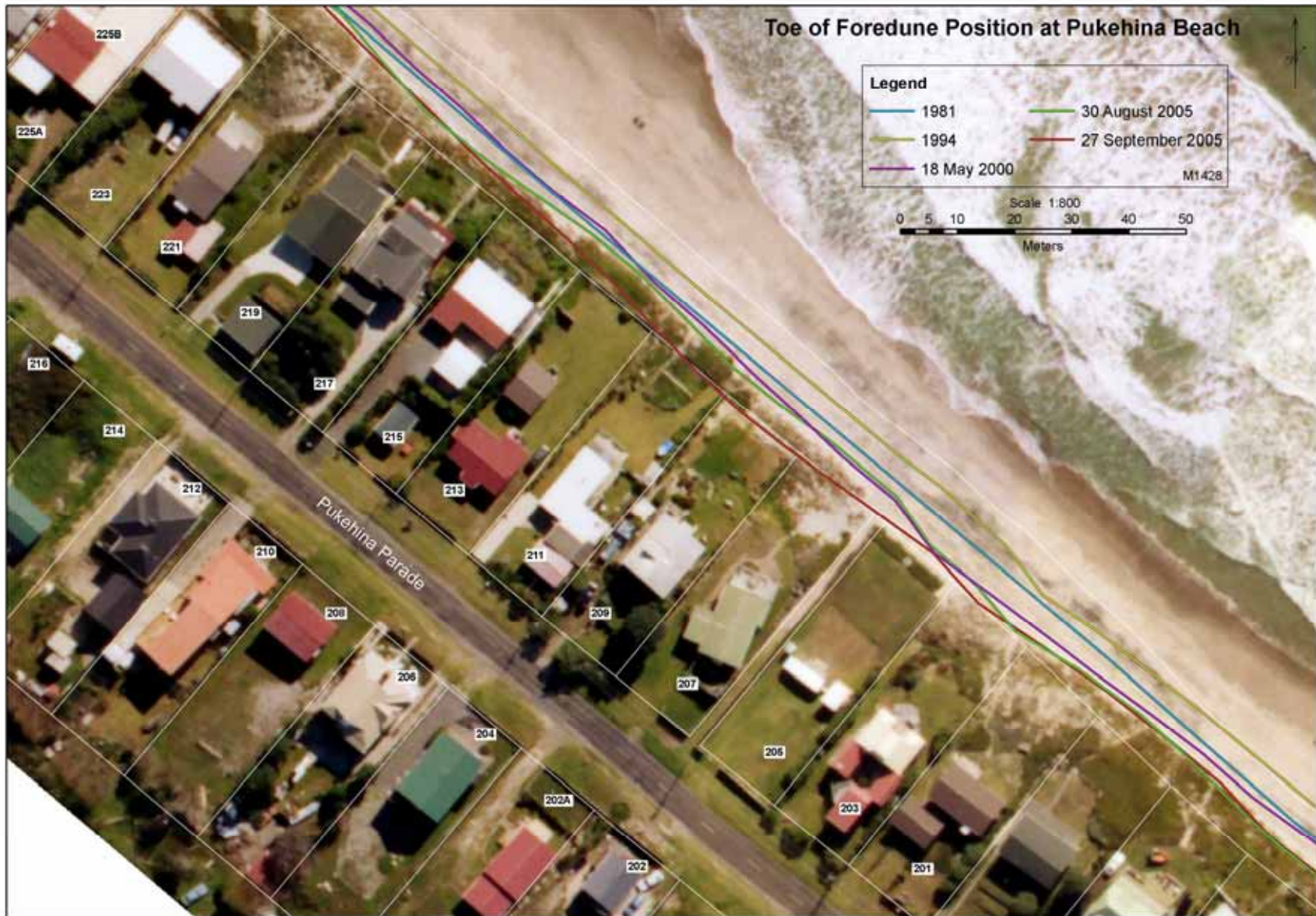
Toe of fore dune position at Pukehina Beach Operations Publication 2008/05
