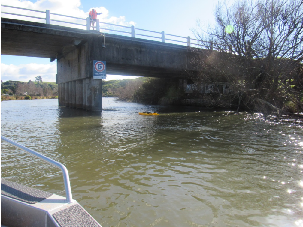
Figure 22 Velocity measuring equipment measuring Ōhau Channel flows at SH33 Bridge.
