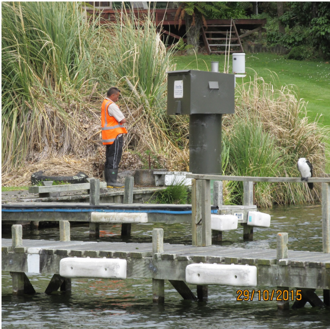
Figure 1 Okawa Bay Lake Level Recorder – Regional Council staff inspecting staff gauge on monthly lake level run.
