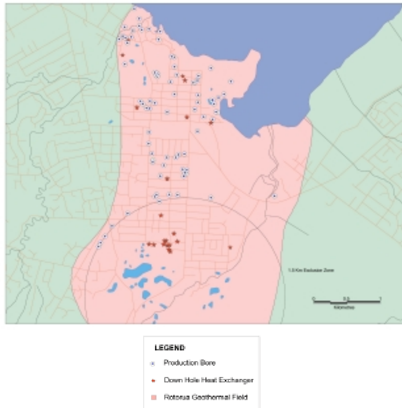
Figure 8.2 Distribution and density of geothermal bores across the Rotorua geothermal field in 1992. Note the use of reinjection and downhole heat exchangers and the absence of production bores within the 1.5 km exclusion zone.
