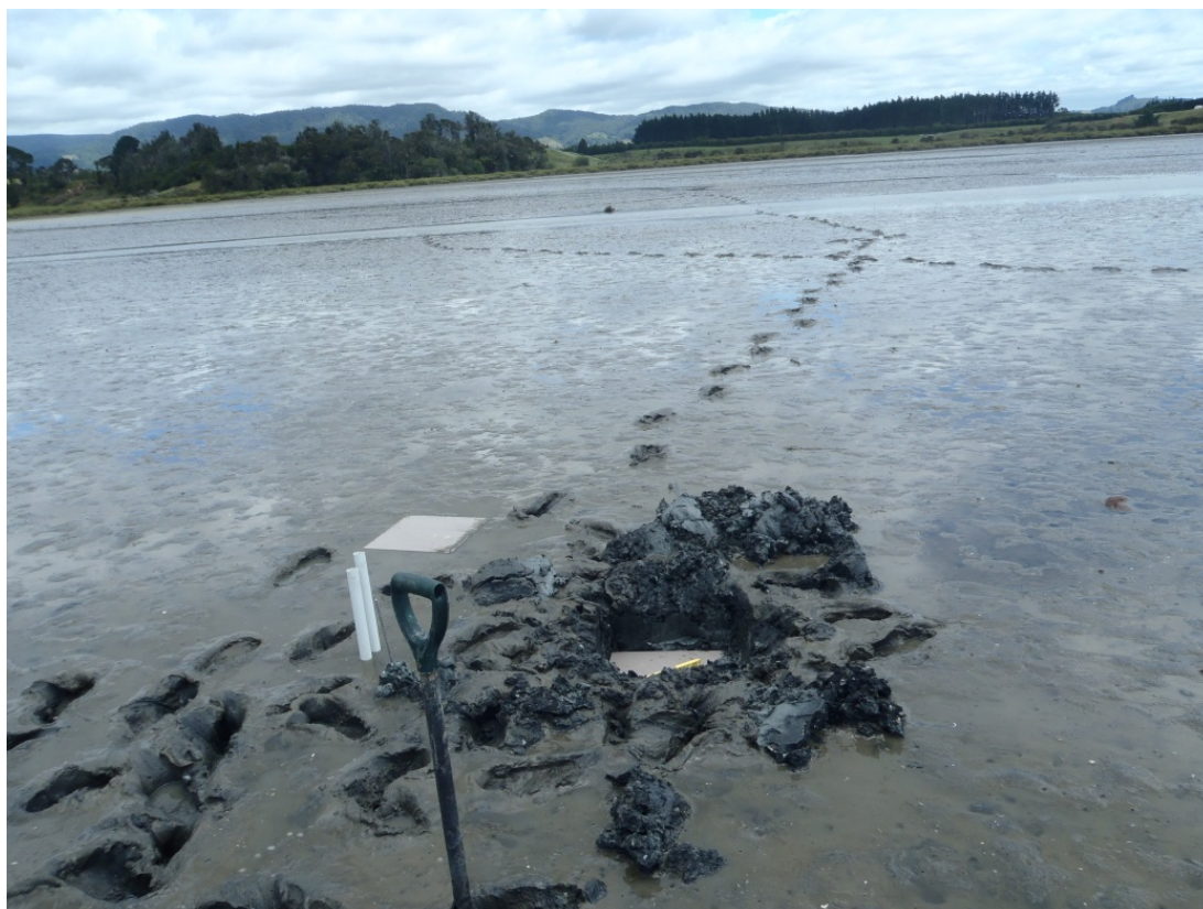
Figure 6 Sediment Accumulation Rate (SAR) monitoring plate installation in Wainui Estuary. Note the thick soft mud anoxic muds a clear sign of high erosion rates from the surrounding catchment.
