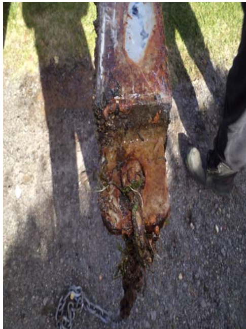
Figures 5 & 6 Following removal, the stop logs were found to be corroded and encrusted with barnacle growth prompting early maintenance to clean, repaint and replace all fittings.
