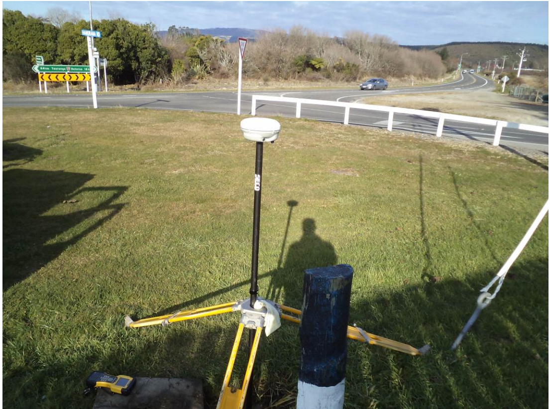
Figure 1 GPS equipment used to establish a Survey Control Network around Rotorua lakes - BM AQ69 at State Highway 33/Hamurana Road turnoff.
