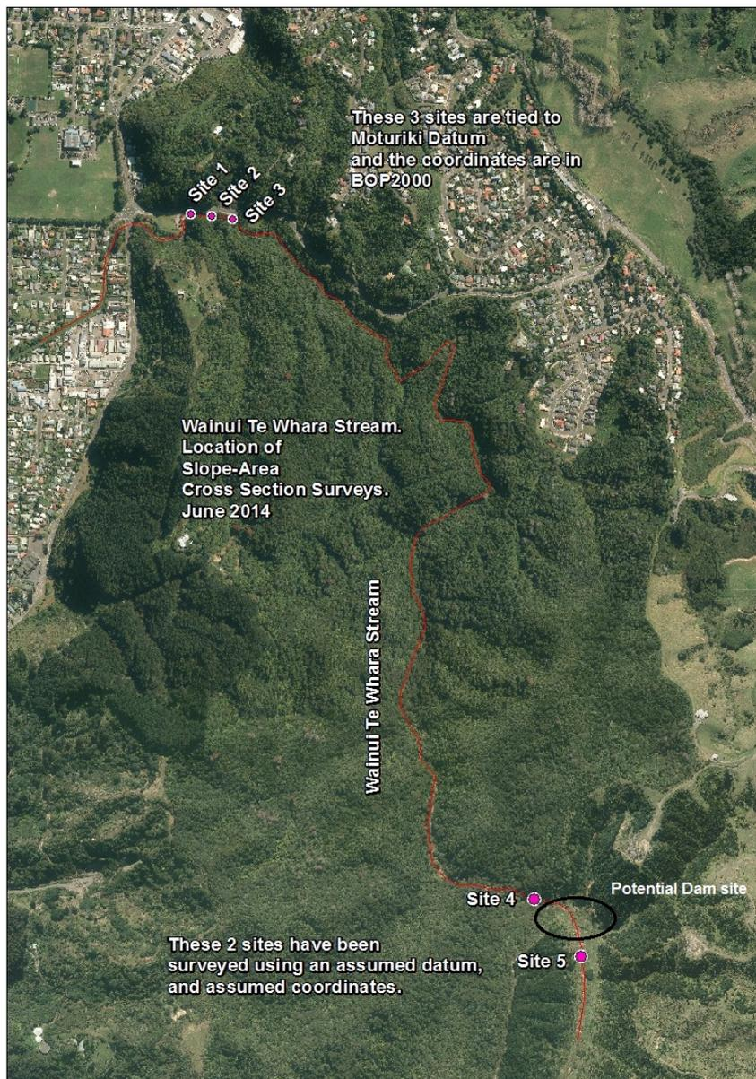
Figure 6 Location of hydraulic analysis sites on Wainui te Whara Stream.
