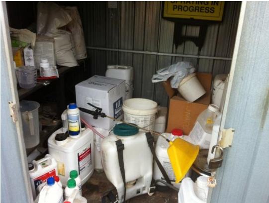
Figure 47 Hazardous substance shed with various chemicals stored without appropriate compartments
