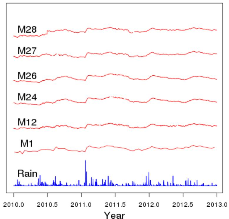
Figure 3.17 Comparison of water levels in the monitor wells M1, M12, M24, M26, M27 and M28 for the period 2010 to 2013. All of these wells penetrate the Rotorua Rhyolite aquifers. The water level variations show clear correlations, despite the wells being widely distributed throughout Rotorua City. The rainfall is scaled to fit onto the figure, but for reference, the highest peak in early 2011 corresponds to 200 mm/day.
