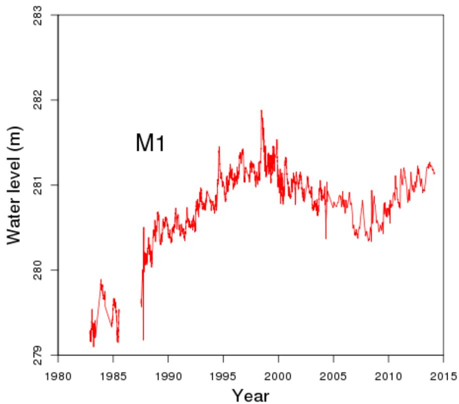
Figure 3.6 Water level in M1, with barometric response removed.
