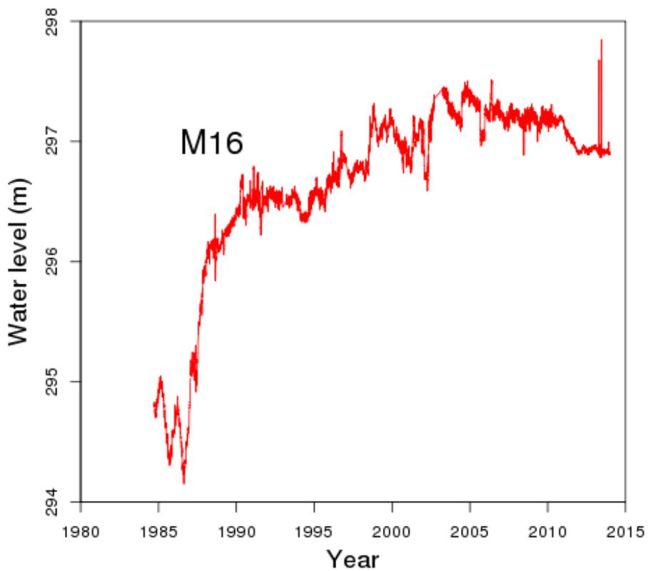
Figure 3.8 Water level for M16, with barometric response removed.
