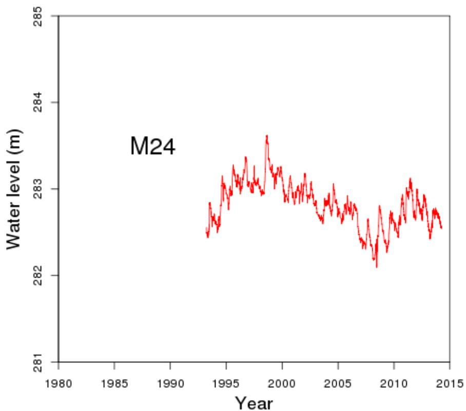
Figure 3.9 Water level for M24, with barometric response removed.
