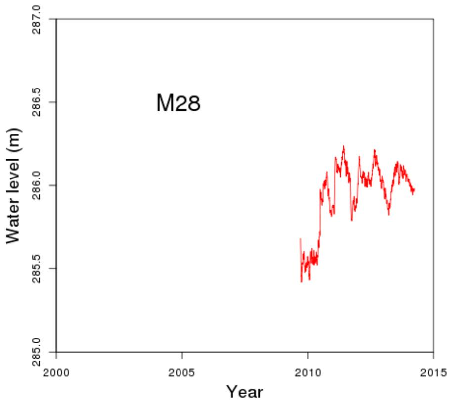
Figure 3.15 Water level in M28, with barometric response removed.
