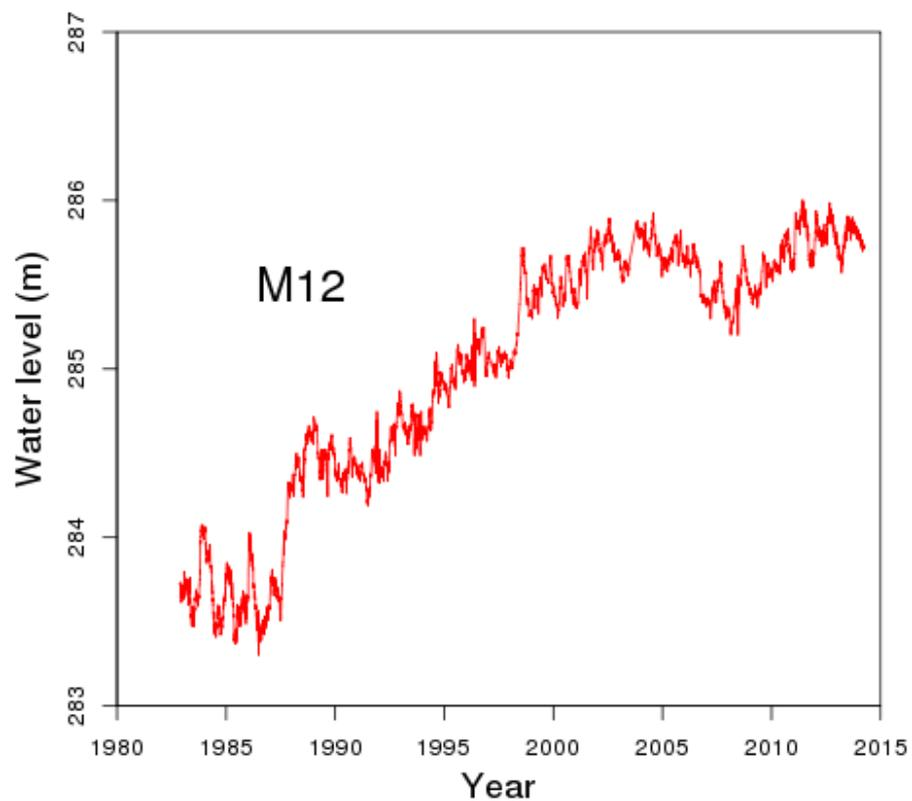
Figure 3.7 Water level for M12, with barometric response removed.
