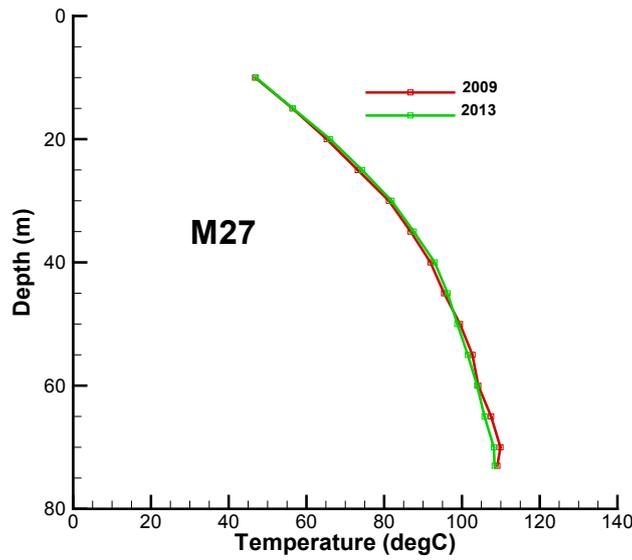
Figure 3.36 Temperature profiles for M27, from 2009 and 2013.
