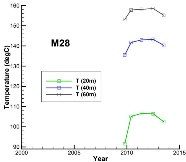
Figure 3.41 M28 temperatures at 20, 40 and 60 m versus time.
