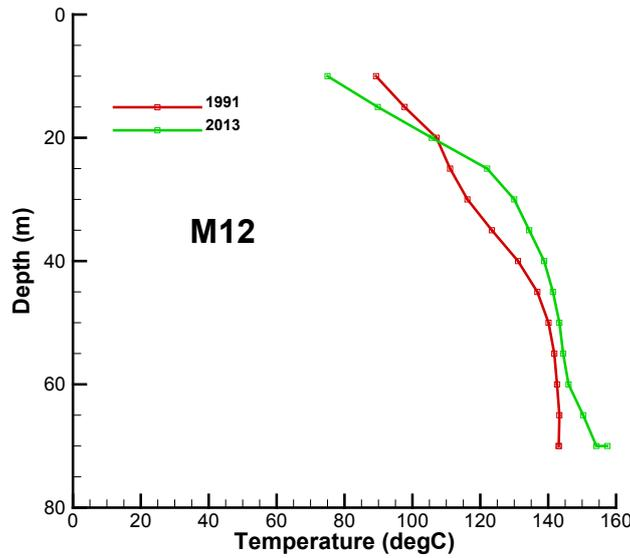
Figure 3.21 Temperature profiles for M12, from 1991 and 2013.
