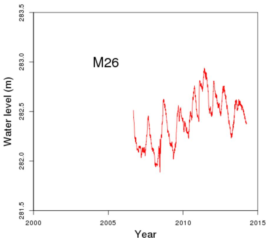
Figure 3.13 Water level in M26, with barometric response removed.
