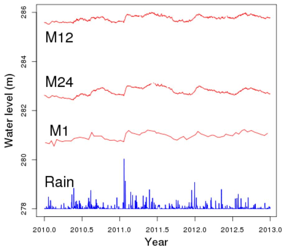
Figure 3.11 Comparison of water levels in M1, M12 and M24 and rainfall for the period 2010 to 2012. The heaviest rainfall event, in early 2011, is coincident with a step change in the water levels of all three wells. The rainfall is scaled to fit onto the figure, but for reference, the highest peak in early 2011 corresponds to 200 mm/day.
