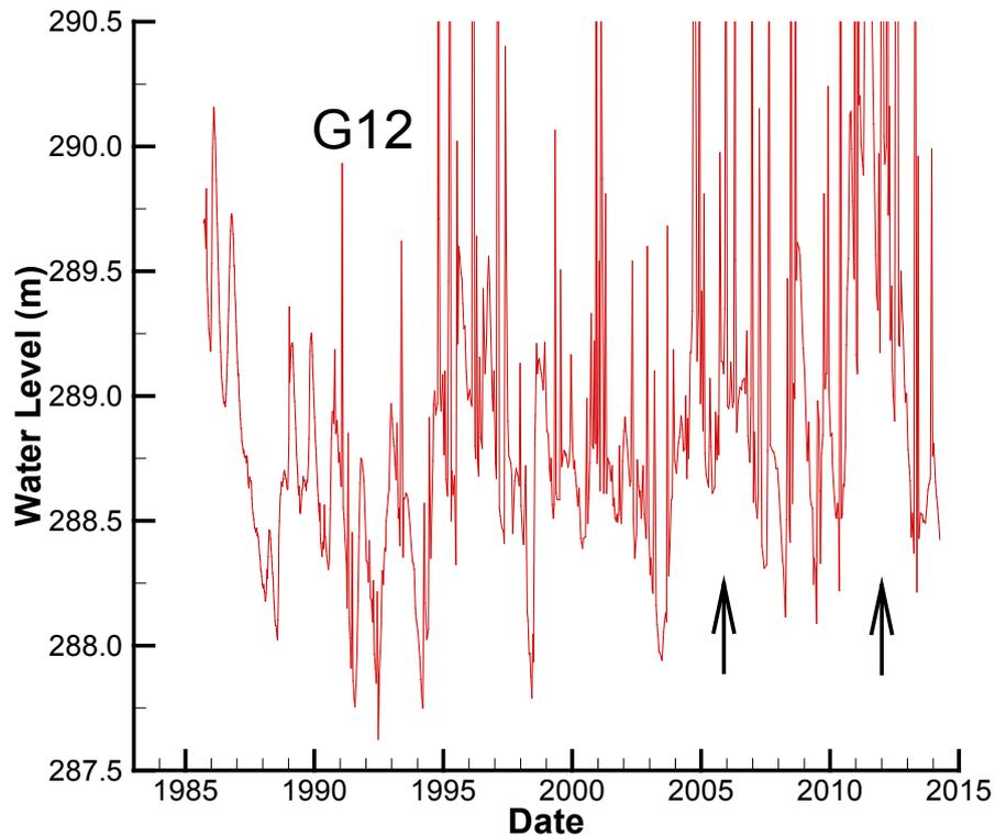
Figure 4.3 Water level in G12, on the same vertical scale as the other G-well plots. The data for G12 contains numerous spikes to above 290.5 m but in this figure has been clipped at to maintain the same vertical scale for all the G-wells plots. The arrows indicate two broad peaks which also occur in G11 and G13.
