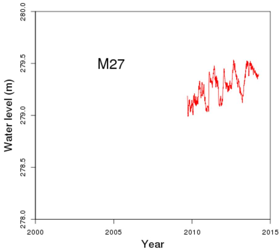
Figure 3.14 Water level in M27, with barometric response removed.
