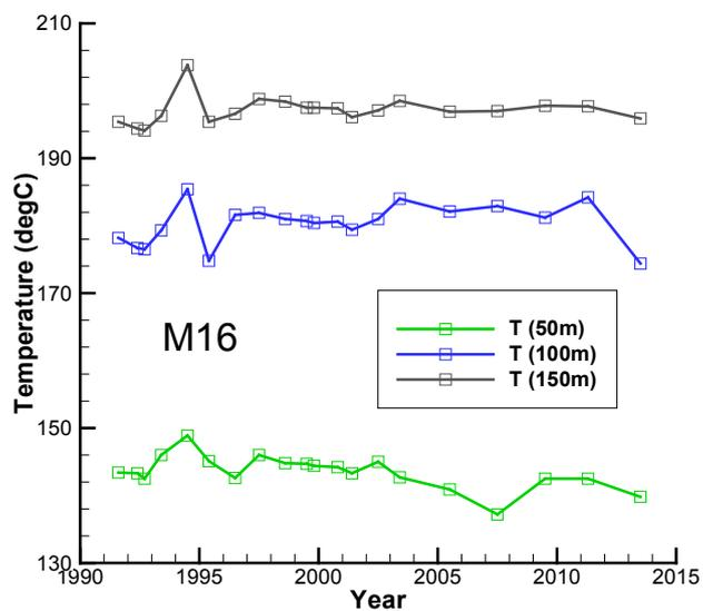
Figure 3.26 M16 temperatures at 50, 100 and 150 m versus time.
