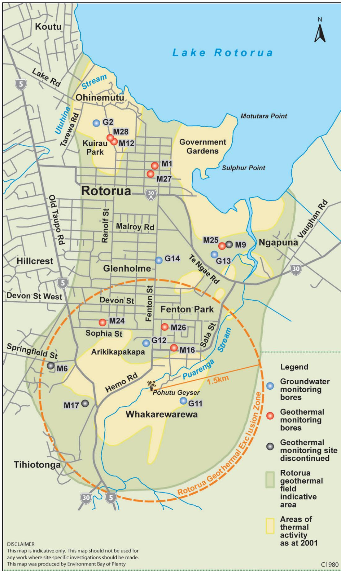
Figure 1.1 Location map showing the positions of monitor wells and shallow groundwater wells at Rotorua. Figure courtesy of Bay of Plenty Regional Council.
