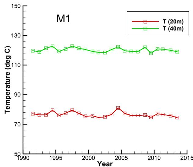
Figure 3.20 M1 temperatures at 20 and 40 m depth versus time.
