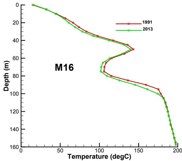
Figure 3.24 Temperature profiles for M16, from 1991 and 2013.
