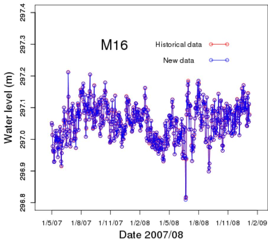
Figure 3.2 Data overlap for M16. The two sets of data show no significant difference over the period of overlap.
