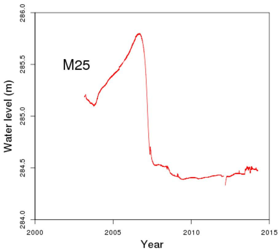
Figure 3.12 Water level for M25, with barometric response removed. The water levels after March 2012 have been adjusted downward by 0.6 m to account for changes in the data following remedial work on the well.
