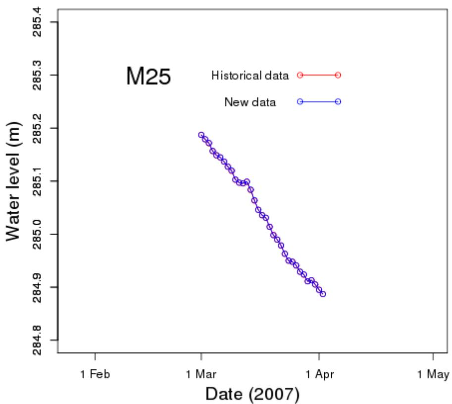
Figure 3.4 Data overlap for M25. The two sets of data show no significant difference over the period of overlap.
