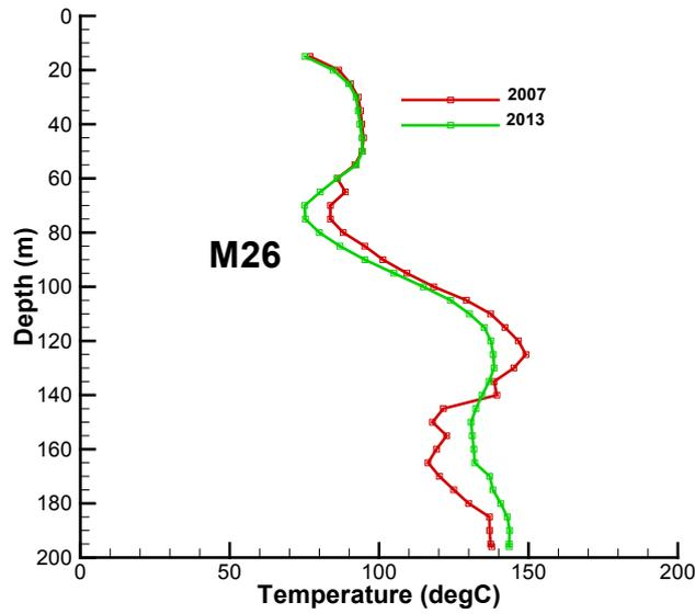
Figure 3.33 Temperature profiles for M26, from 2007 and 2013.
