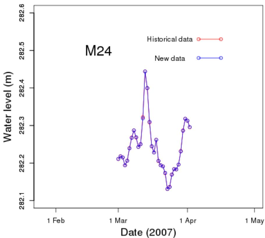
Figure 3.3 Data overlap for M24. The two sets of data show no significant difference over the period of overlap.
