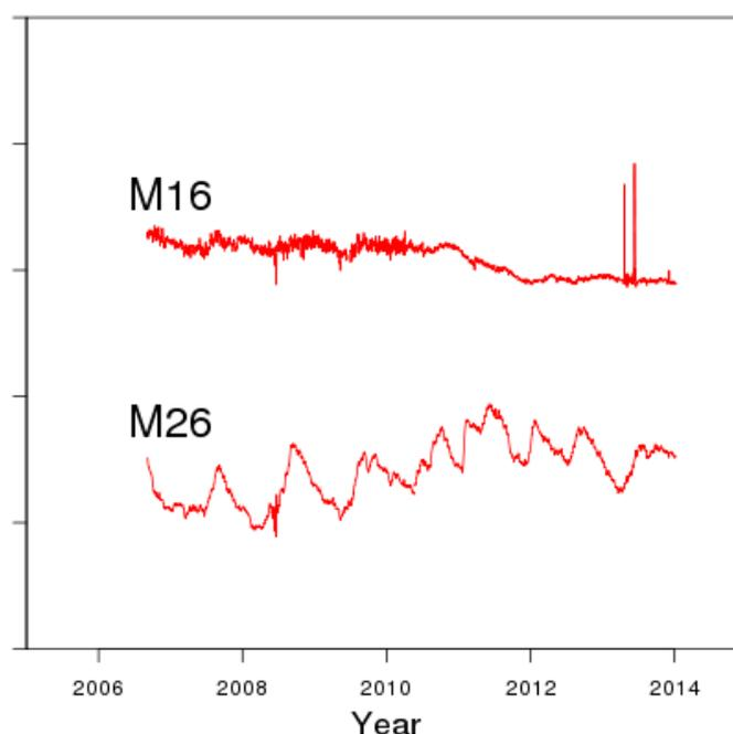
Figure 3.42 Comparison of water levels in M16 and M26. For scale, the tick marks on the vertical axis are 1 m apart.
