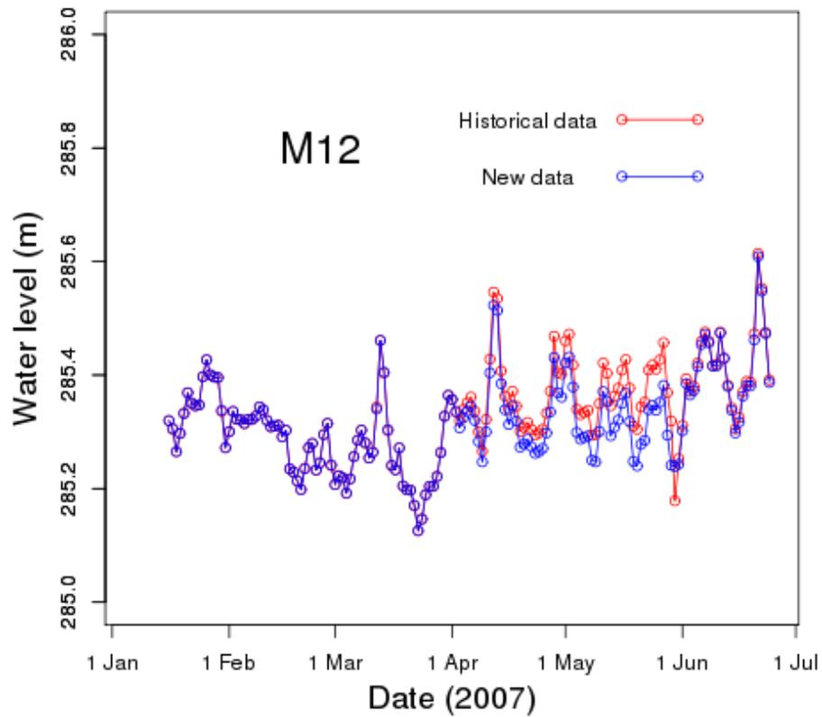
Figure 3.1 Data overlap for M12. The two sets of data show a difference of up to about 0.03 m between early April and late May 2007.
