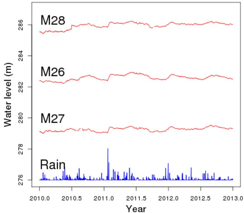
Figure 3.16 Comparison of water levels in M26, M27 and M28 and rainfall for the period 2010 to 2012. The heaviest rainfall event, in early 2011, produces a noticeable change in the water levels of all three wells. The rainfall is scaled to fit onto the figure, but for reference, the highest peak in early 2011 corresponds to 200 mm/day.
