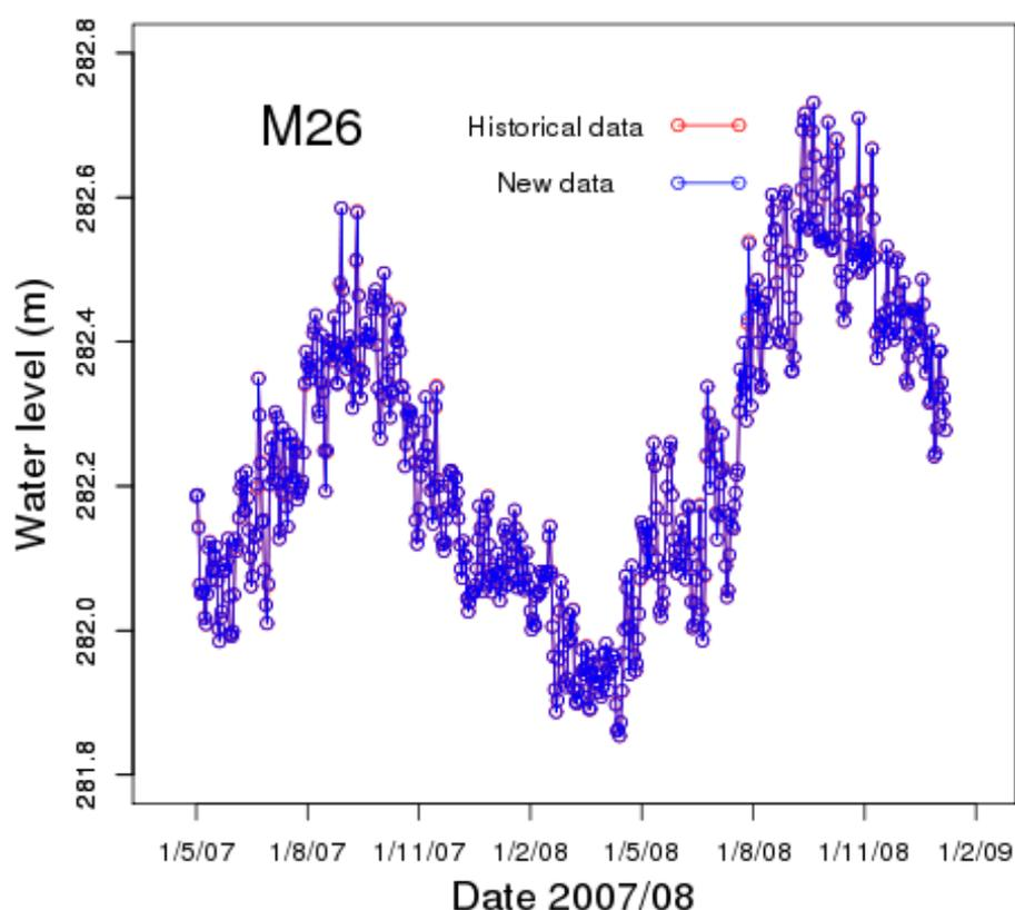
Figure 3.5 Data overlap for M26. The two sets of data show no significant difference over the period of overlap.
