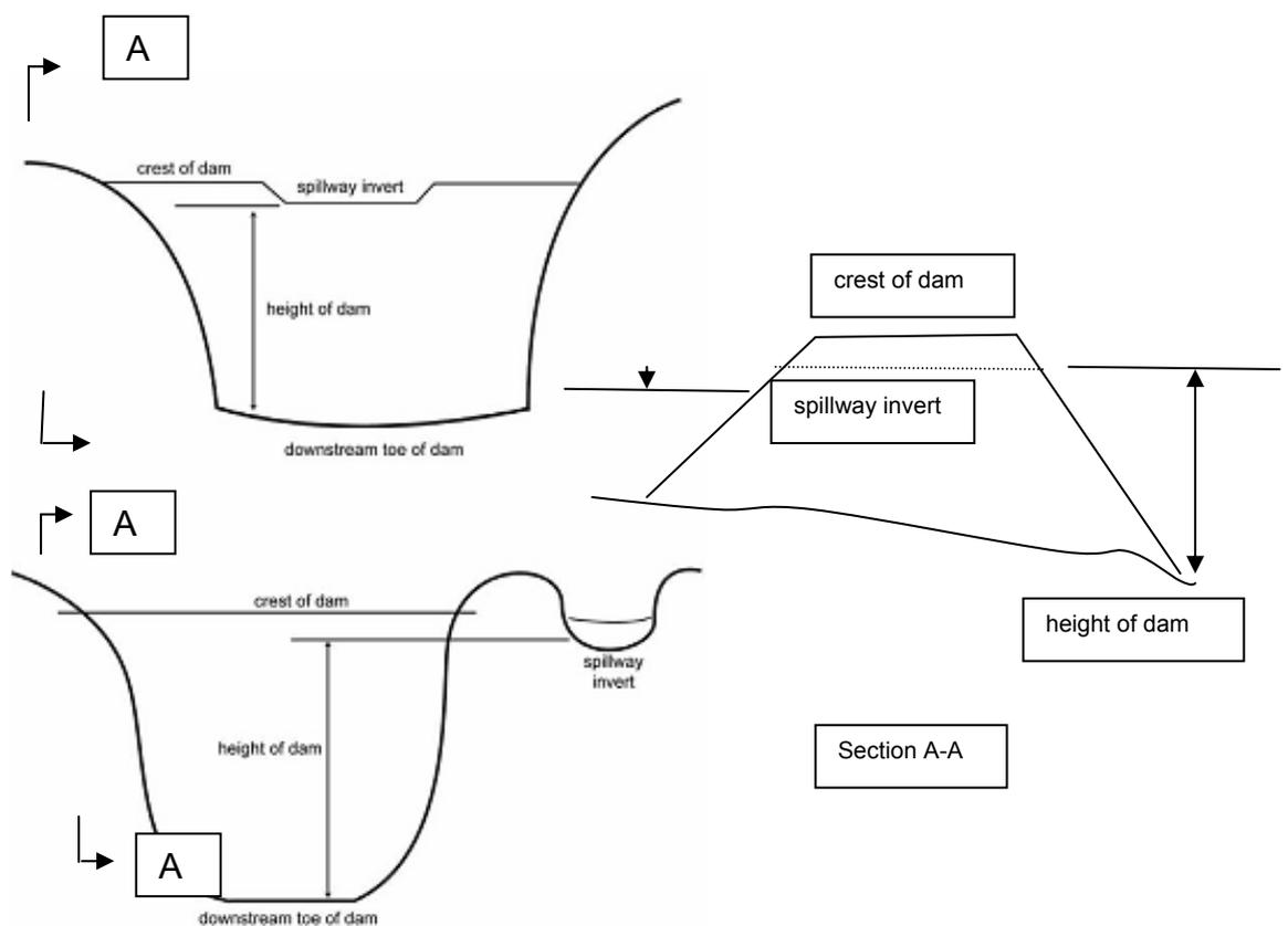
*Figure 4.1 Cross-section of a typical small dam defining measurement of the dam water retention height (Source: Regional Water and Land Plan, Bay of Plenty Regional Council, 2008).*
