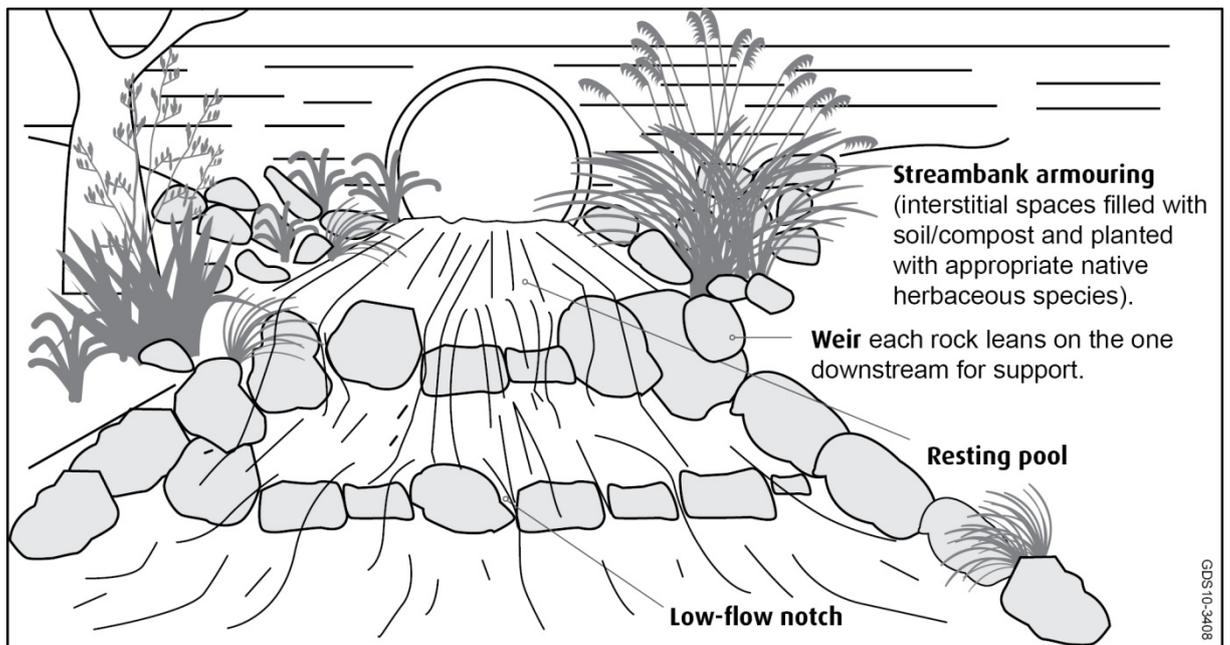
A succession of weirs helps raise the water level so it creates an impoundment through the culvert.
