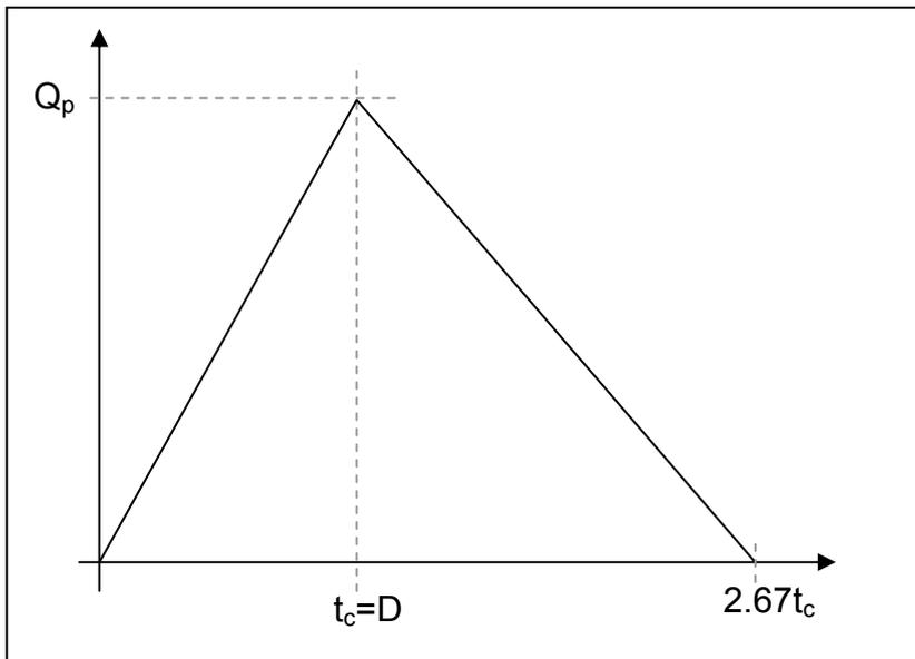
Figure 5.1 Simple hydrograph for storm flow
