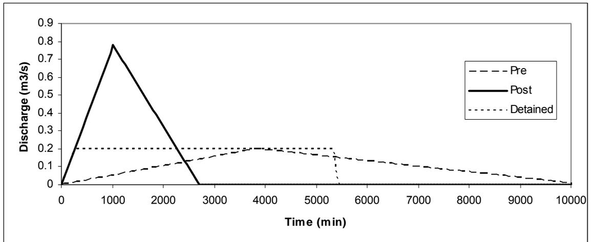
Figure 5.2 Sample Pre-, Post- and Detained hydrographs
