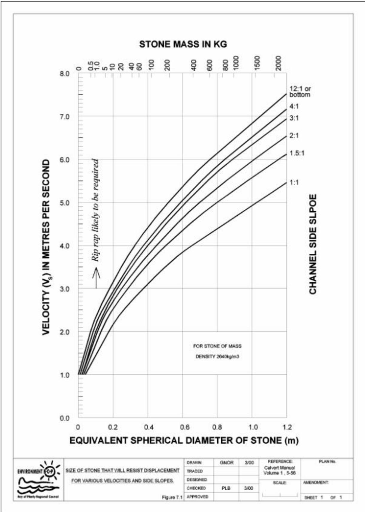
Figure 7.1 Rip-rap sizing diagram to determine  $d_{50}$
