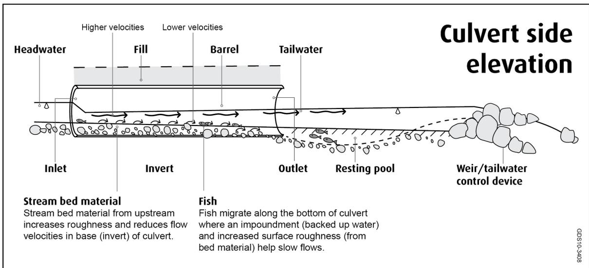
Figure 7.3 Culvert details suitable for fish passage
