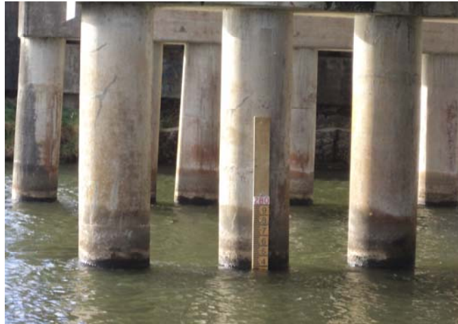
Figure 9 New Ohau Channel/State Highway 33 Staff Gauge located on pillars of State Highway 33 Bridge at Mourea.
