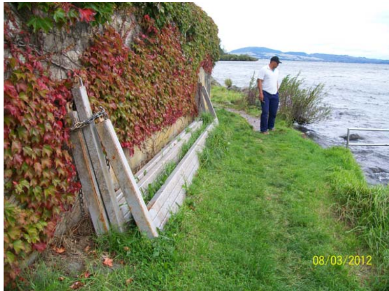
Figure 4 Ohau Weir Stop logs (x3) stored onsite after removal (dimensions 6m x 0.3 m).
