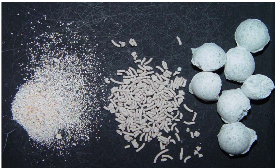
Figure 1. Media tested in this study, from left to right, treated zeolite, Phoslock , and Baraclear .
